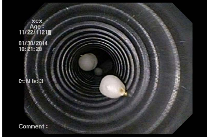
Figure 2-7: Custom tubular structure that emulates the tract with spheres of known sizes that simulate polyps.
