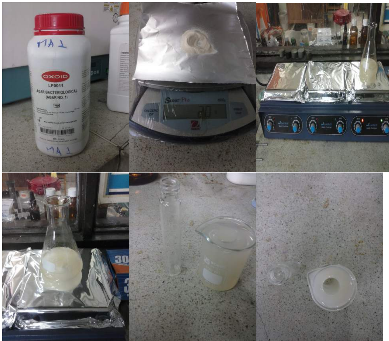
Figure 6.5: Process of elaboration of a prototype agar phantom.
