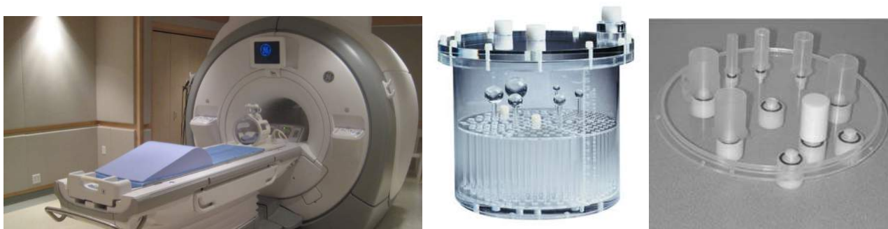
Figure 6.2: Experimental design for the acquisition of PET-CT images from the phantom Jaszczak (central image). Taken from [37].
