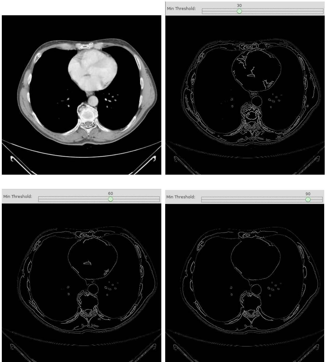
Figure 7.26: CT Test Image (upper left), and Canny Edge detection with different minimum threshold.
