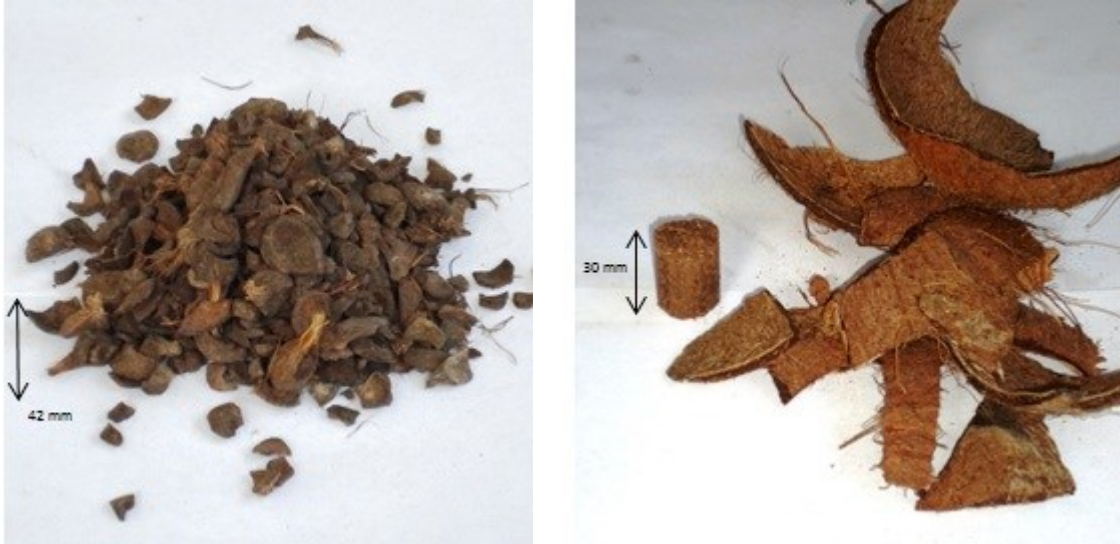
Figure III-1 Samples of oil palm shells (left) and Coconut shells (right) as received
