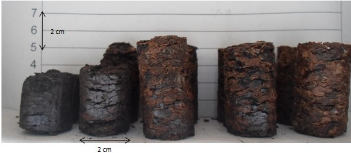
Figure V-2 Coal-cocoa pellets made from intermediate particle size and organized by the cocoa content in the blend (0, 30, 50, 70 and 100%wt)
