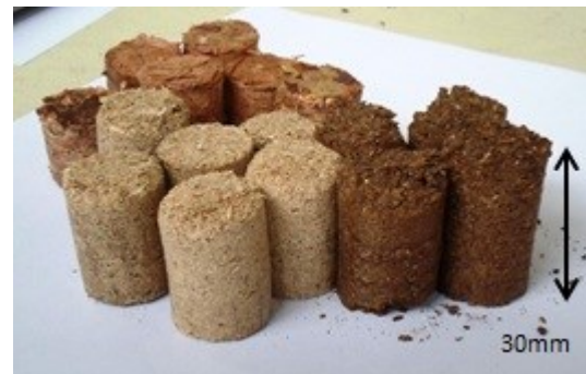
Figure III-3 Pellets made from sawdust, coconut shells, and wood shavings.
