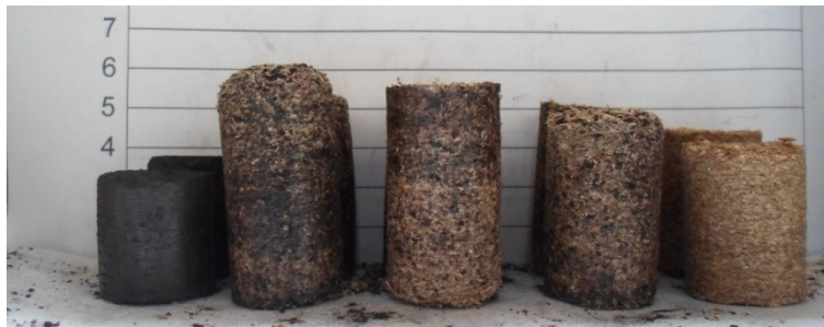
Figure IV-2 Pellets made from sawdust-coal mixtures, varying sawdust content in the mixture (0, 30, 50, 70, and 100%wt from left to right), and particle size between 1.19 and 0.297 mm
