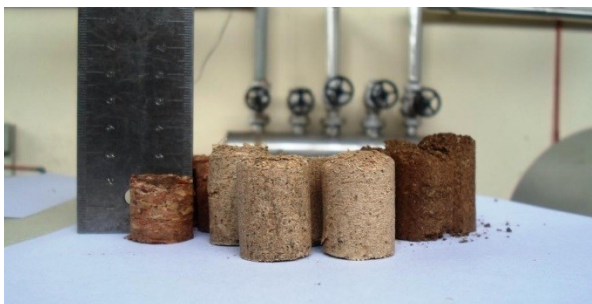
Figure III-3 Pellets made from sawdust, coconut shells, and wood shavings.
