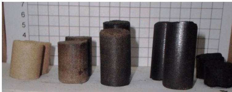
Figure IV-3 Pellets made from sawdust-coal mixtures, varying sawdust content (100, 70, 50, 30, 0wt from left to right) and using fine grinds with particle size <0.297 mm
