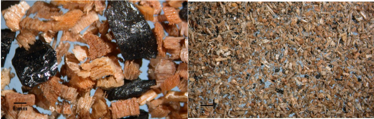
Figure IV-6 Optical microscopic images of sawdust coal mixtures (Ics-50/50 and Fcs-50/50) before pressing. Left exhibits particle size in the range of 4.76-1.19mm; whereas right shows particle size smaller than 0.297mm
