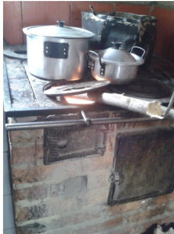
Figure IV-1 Typical household cooking stove fed with coal and wood in Cundinamarca and Boyaca areas
