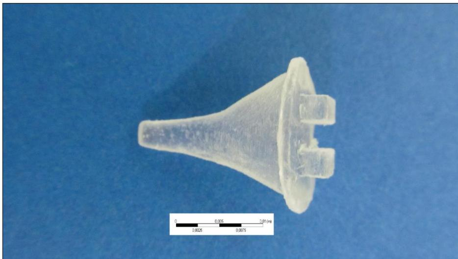
**Figura 3-57:** Prototipo del vástago del metacarpo
