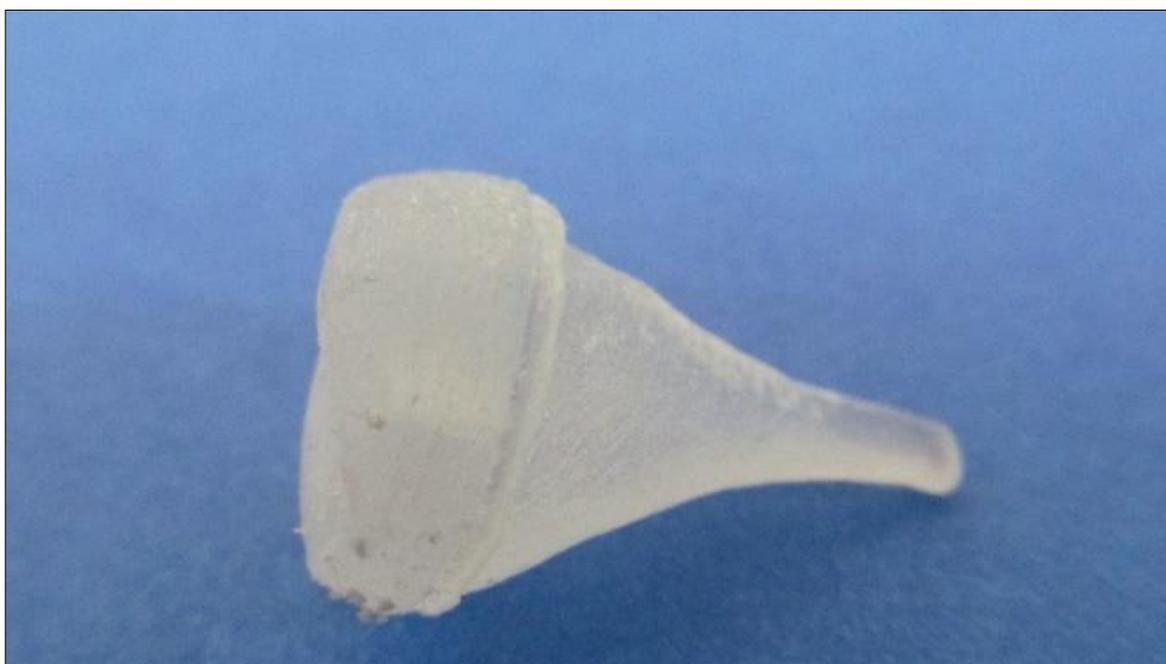
**Figura 3-61:** Ensamble vástago-cabeza para el metacarpo
