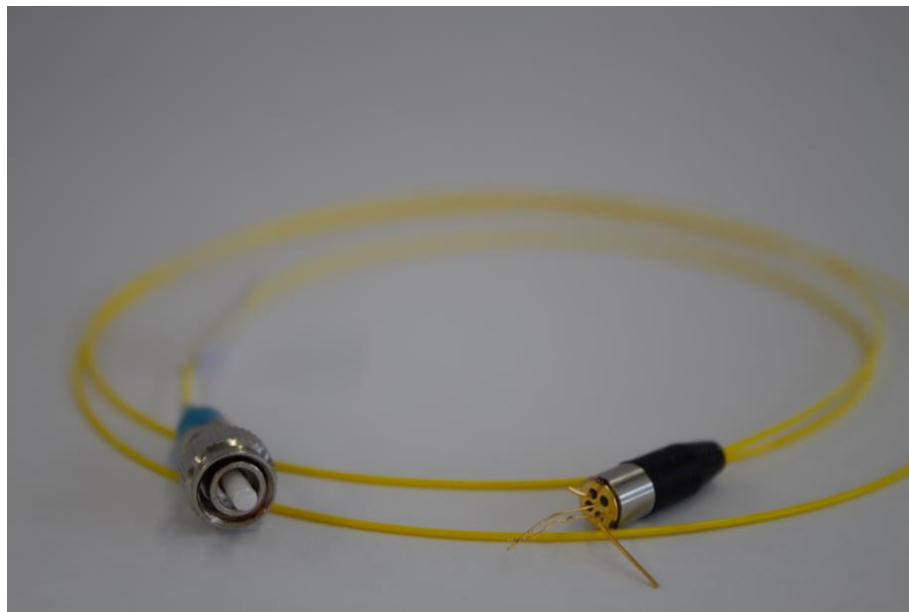
Figure 14 Raycan pigtailed VCSEL.
