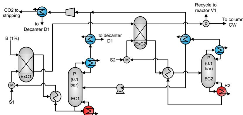
Figure 3-4. Dual extraction configuration studied in this work
