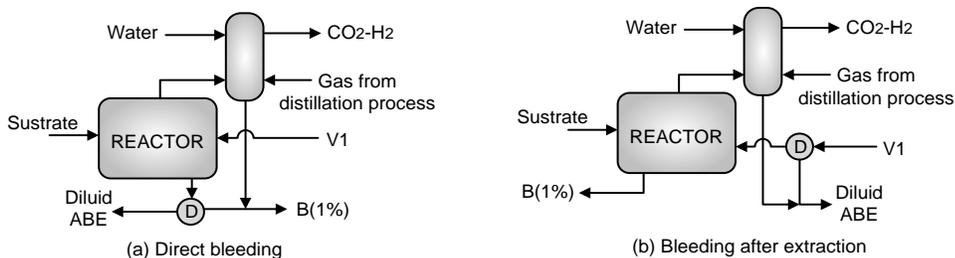
Figure 3-2. Alternatives of bleeding in external extractive fermentation
