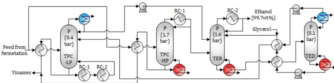
Figure 1-6. Scheme IV (S-IV): double-effect extractive distillation by ethanol dehydration
