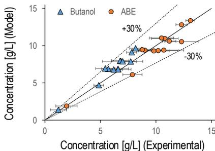
Figure 5-2. Parity diagram of butanol and ABE prediction by kinetic model. Experimental data from Zheng et al. <sup>153</sup>
