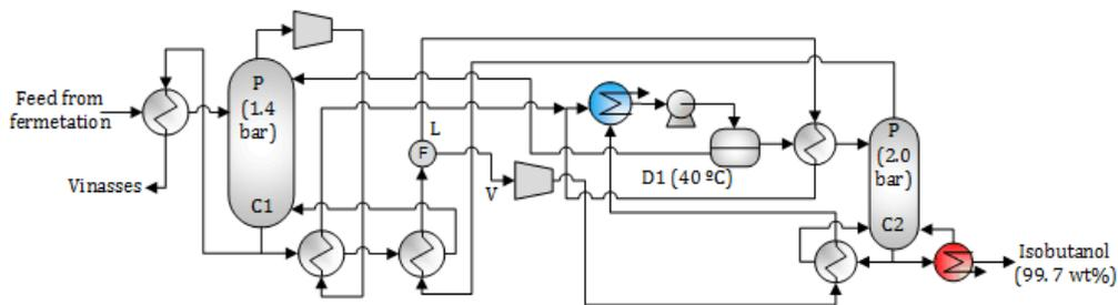
Figure 1-2. Scheme proposed of integrated distillation vapor compression for isobutanol dehydration (S-I)
