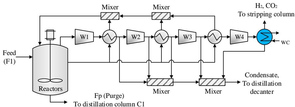
Figure 4-1. Simultaneous fermentation, saccharification and flash evaporation with a heat pump (SFS-V) proposed with 2-stage condensing
