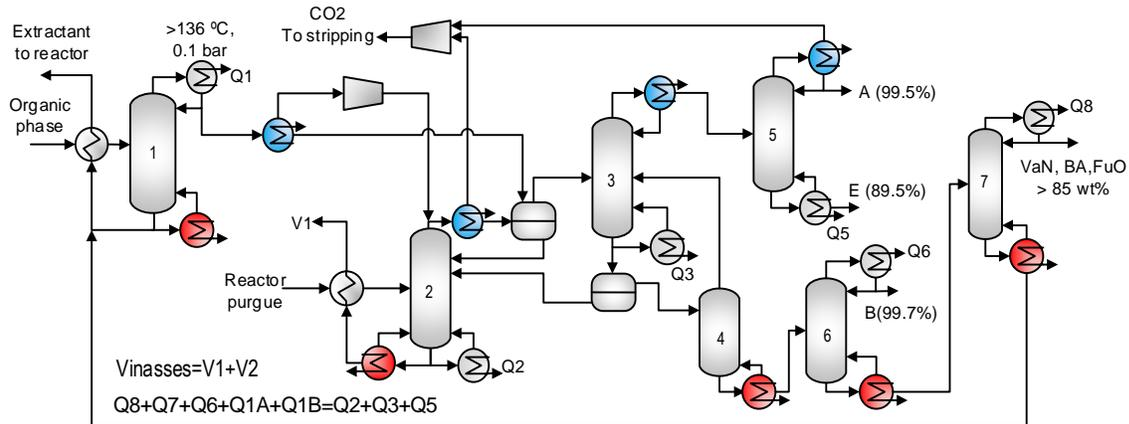
Figure 5-4. Distillation system with partial OAL loss in the top of extractant regeneration column and heat integration
