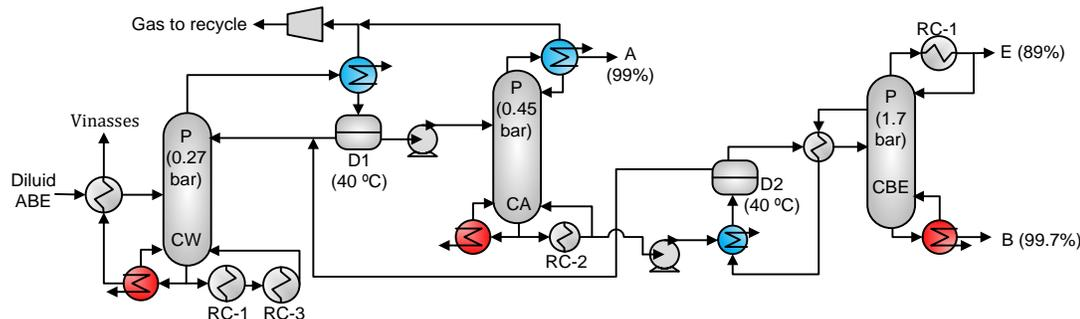
Figure 3-1. End recovery scheme proposed in this work to ABE purification
