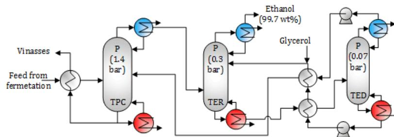
Figure 1-4. Ethanol separation by conventional extractive distillation (C-1)
