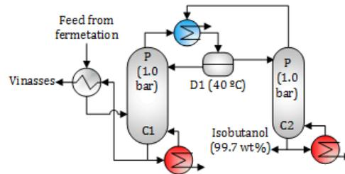
Figure 1-1. Isobutanol separation by conventional distillation
