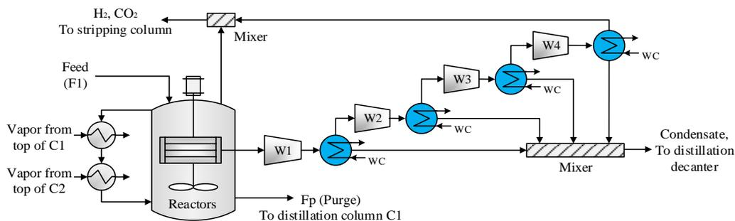
Figure 4-2. Production scheme with simultaneous fermentation, saccharification and pervaporation (SFS-P)
