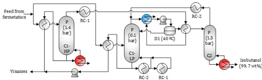
Figure 1-3. Scheme proposed by isobutanol separation with double-effect distillation (S-II)
