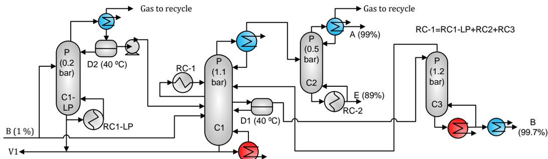
Figure 2-7. Configuration with 4 distillation columns and double effect integration (4DC-DE)
