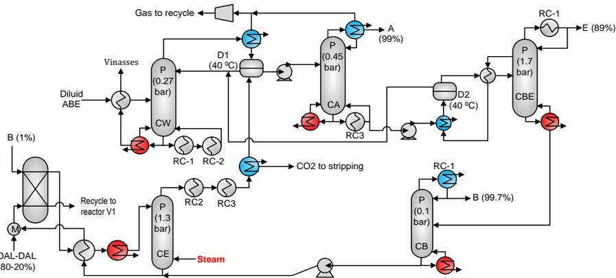
Figura 3-7. Steam direct regeneration using mixed extractants (OAL-DAL)
