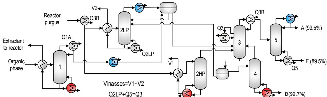
Figure 5-3. Distillation system with extractant regeneration to vacuum and double-effect heat integration
