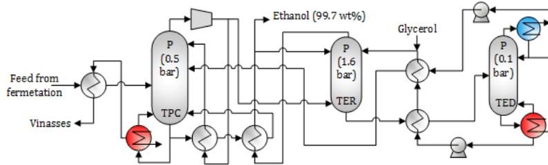
Figure 1-5. Scheme proposed by ethanol dehydration with vapor compression (S-III)
