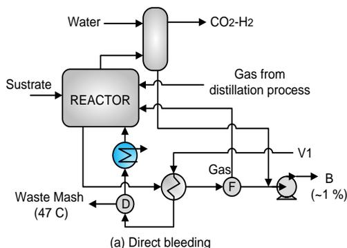
Figure 2-2. Fermenter with stillage recycle
