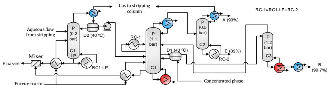
Figure 4-3. Scheme of multifect-distillation by acetone, ethanol, and butanol purification (S-I)
