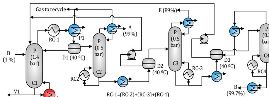
Figure 2-3. Heat-integrated configuration with 4 distillation columns (4DC) proposed by ABE recovery
