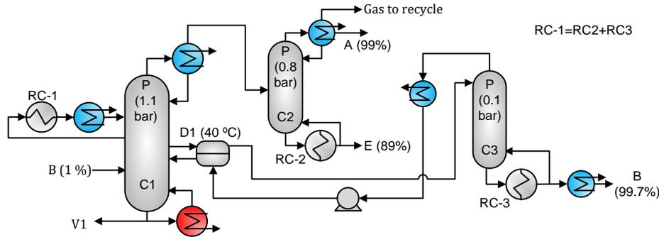
Figure 2-5. Scheme with 3 distillation columns (3DC)
