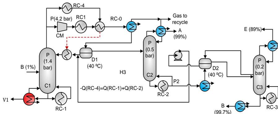
Figure 2-6. Configuration with 3 distillation columns and vapor compression (3DC-VC)
