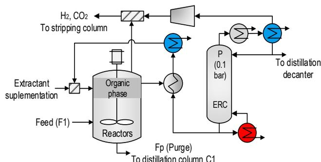
Figure 5-1 Integrated reactor with liquid extraction system
