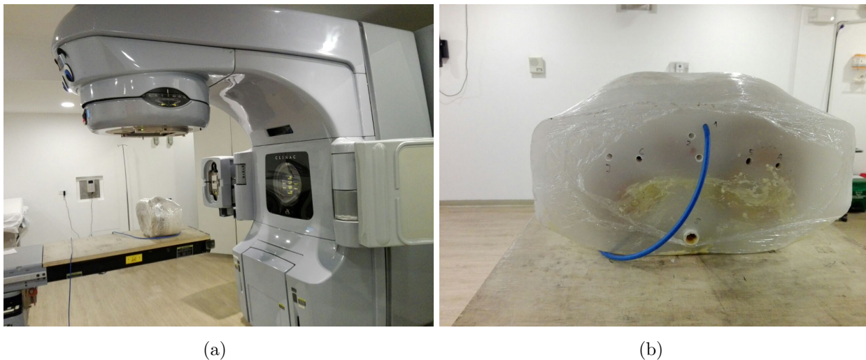
Figure 4-27.: Experimental setup for the measurement of the absolute dose in the thorax phantom. a) View of the phantom place on the table of the linear accelerator and b) the phantom with its holes and the ionization chamber.
