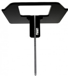
Figure 3-14.: Front Pointer device for SSD measurement [5].
