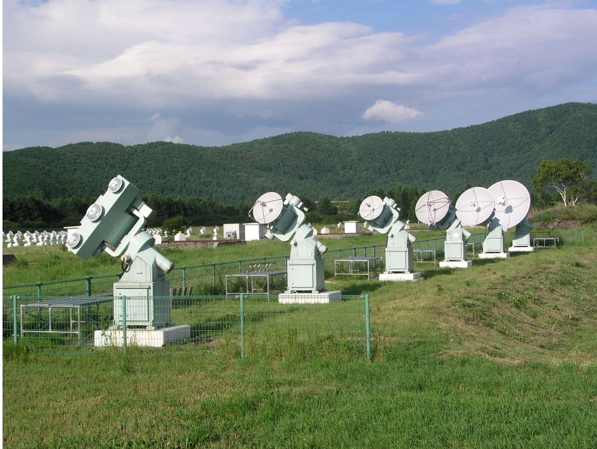
Figure 3-2.: Configuration of the Nobeyama Radio Polarimeters at the NRO 2 . The furthest plate corresponds to the detector at 1GHz. The smallest the plate diameter, the highest is the frequency observed. The nearest mount has three plates. Those of the edges registers solar signals at 80GHz, while the one at the center measures at 35 GHz.
