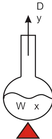
Figure 4.5: Residue curve map experimental set up
