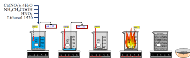
Figure 2-4. Solution combustion synthesis procedure
