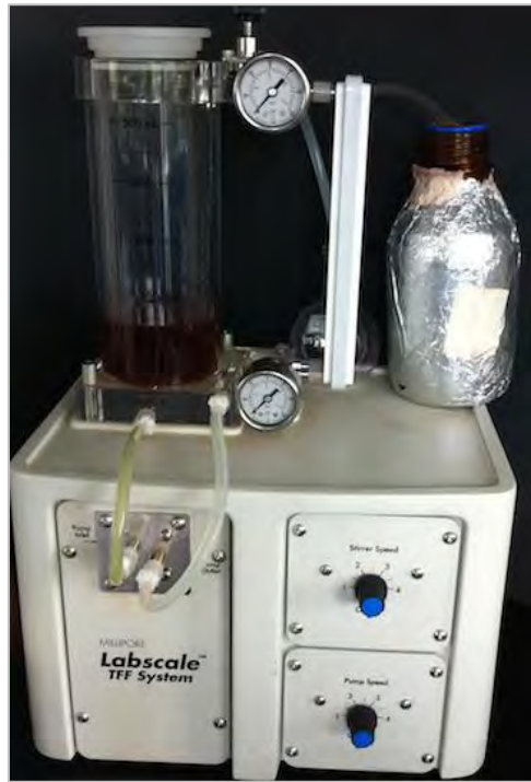
Figure 3.15. Ultrafiltration process for concentrated extracts
