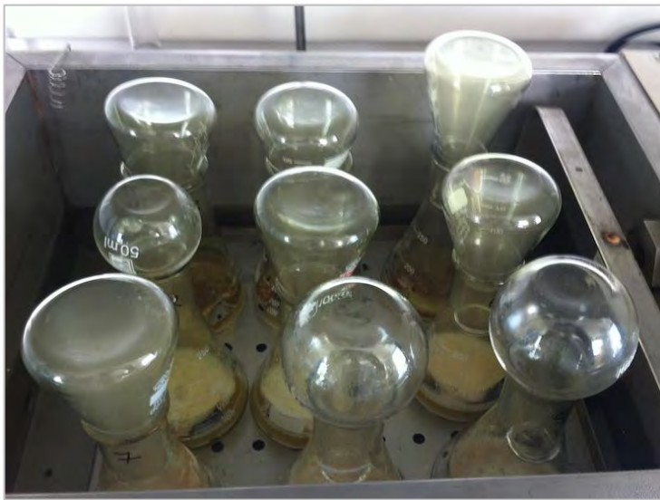
Figure 3.4. Delignification process for holocellulose measurement
