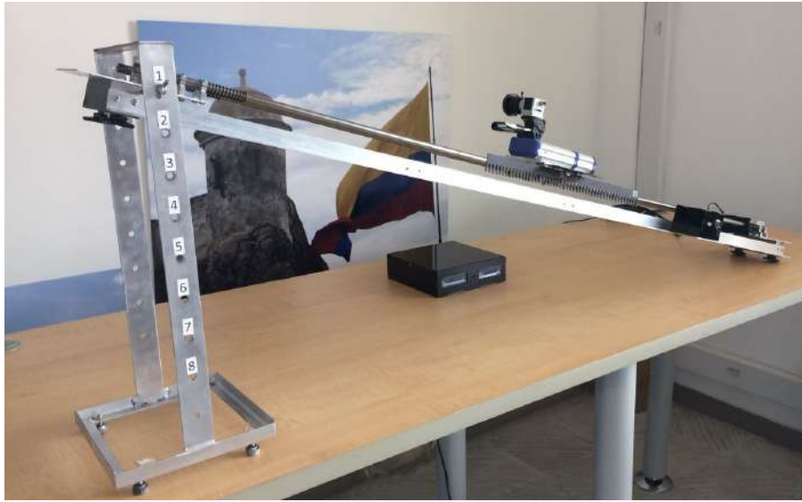
Figure 8.15: Actual electromechanical acceleration system.
