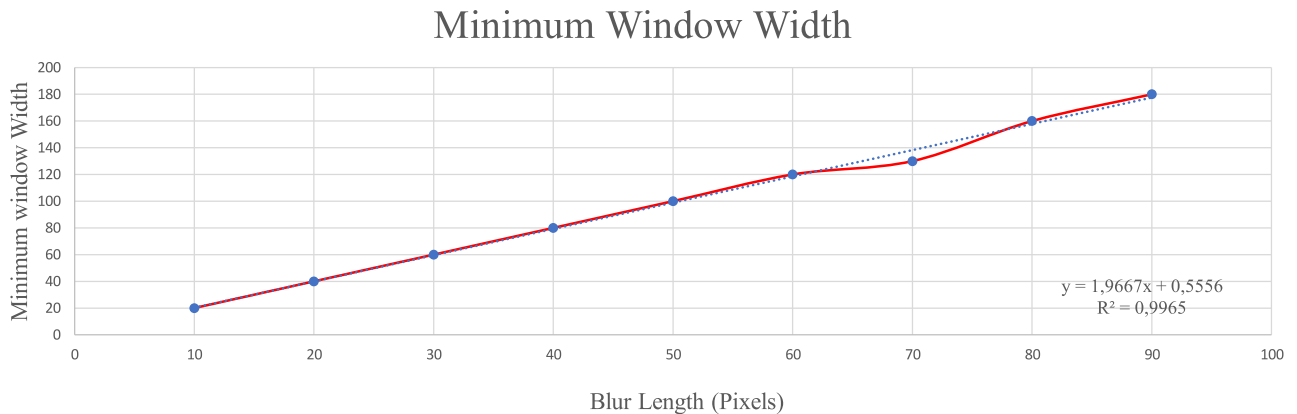
Figure 7.17: Window width that produces minimum error. The window width must be at least the double of the of the blur length.
