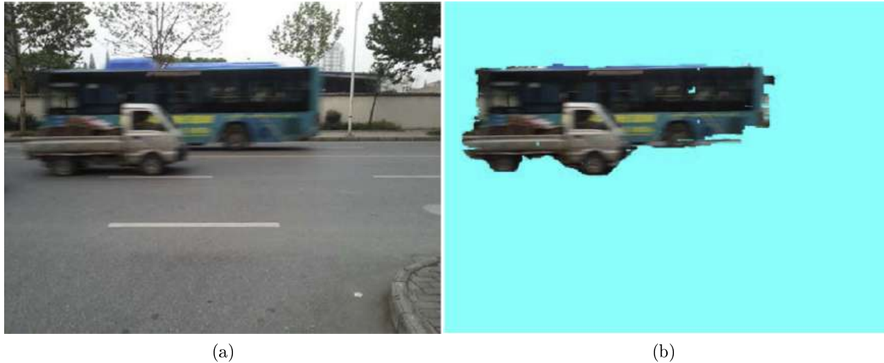
Figure 7.2: Segmentation for real images based on Zhou algorithm [Zhou and Zhang(2018)]. (a) Variant motion blur image with fixed background and vehicles in motion. (b) Segmentation result of image shown in (a).
