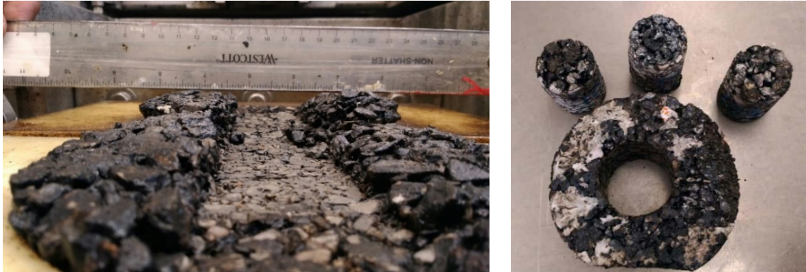
Fig. 3-16. Location of 50mm diameter cores from HWTT samples.
