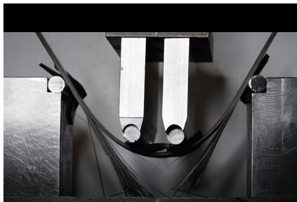
Figure 7-16.: Failure mode in the four-point bending test of Layup B.
