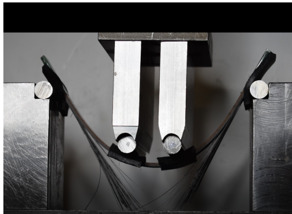
Figure 7-15.: Failure mode in the four-point bending test of Layup A.
