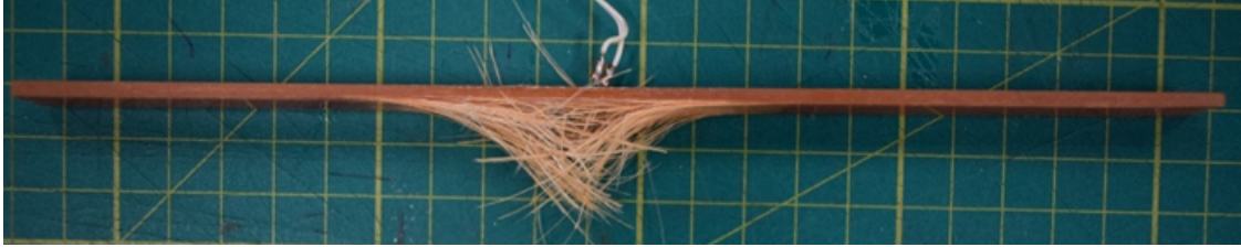
Figure 9-9.: Failure in SGlass specimen with strain gauge.
