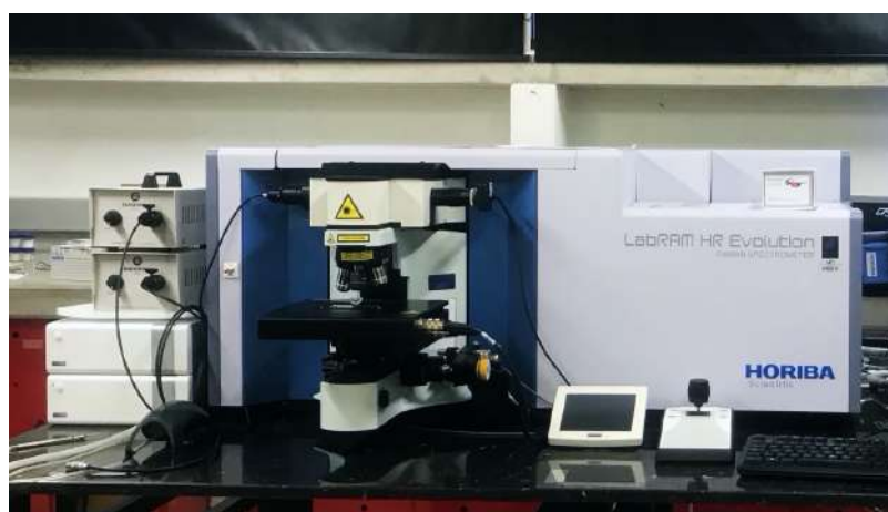
Figura 4-24: Microscopio Raman Confocal Horiba LabRam HR Evolution.
