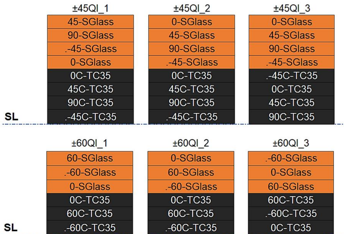
Figure 35 QI layups proposed to understand the interaction between the layers (SL: Symmetric Line).
