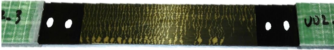
Figure 15 Damage pattern for thin ply hybrid composite [SG/C 2 /SG]s, own source.
