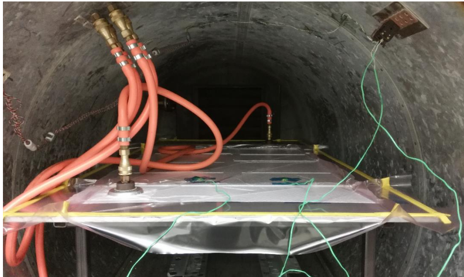
Figure 36 Manufacturing process using an autoclave.
