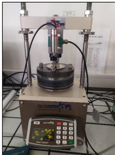
Figure 4-13. Oedometer test in Automatic oedometer system of Global Digital Systems GDS.
