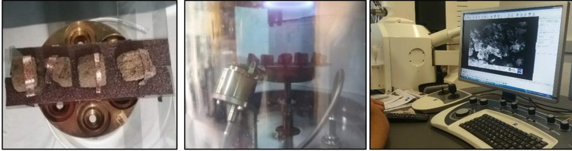
Figure 4-8. Sample preparation for SEM. Left: Geometry samples and putting the sample in the slides. Right: Sputter coating process.
