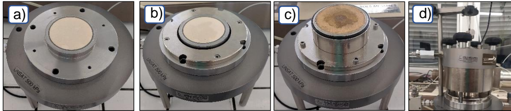
Figure 4-19. Procedure to assemble the equipment a) sample base b) sample base and ring clamp c) assemble the sample d) assemble the part superior to the cell.
