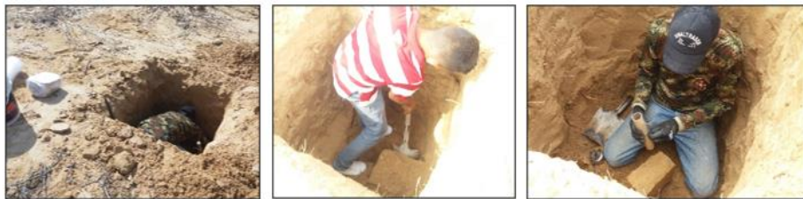
Figure 4-2. Procedure for cubical block sampling of eolian soils.
