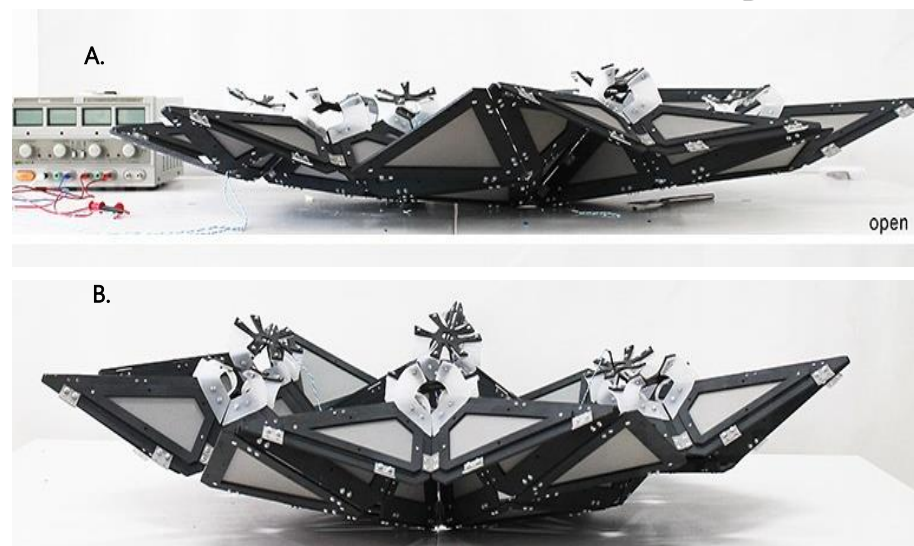
Fig. 35. Translated geometries. Standing structure actuated by SMP. A. open position B. closed position [119].
