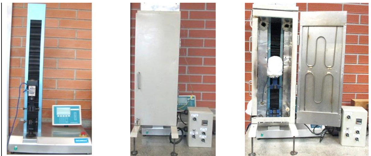
Fig. 43 Customize forced convection thermal chamber with temperature controller
