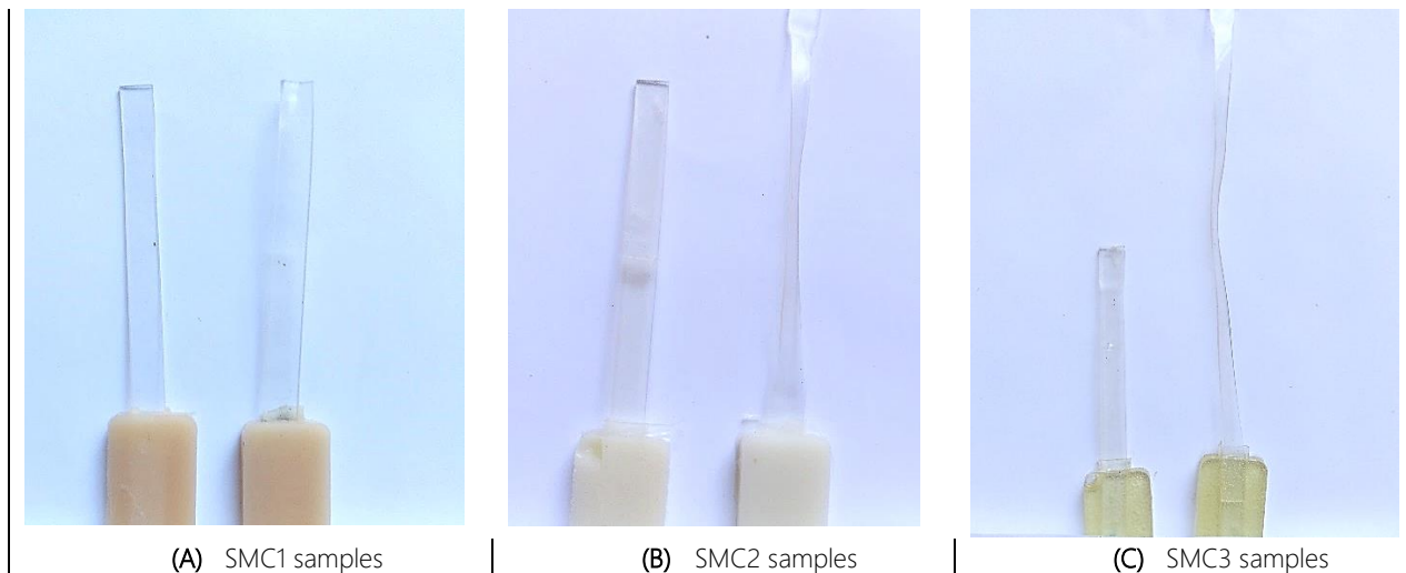
Fig. 73 T-peel after test samples. Left as-received, right treated
