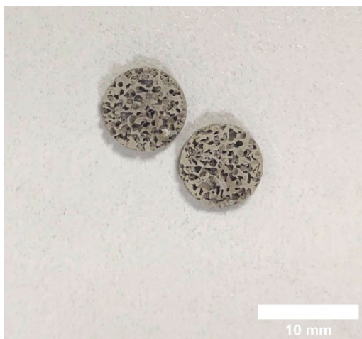
Figure 3-1. Photograph of the AZ31-based scaffolds obtained via infiltration casting.
