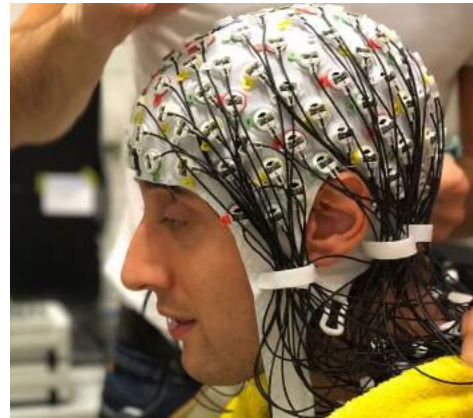
(b) hdEEG helmet with 128 electrodes.
