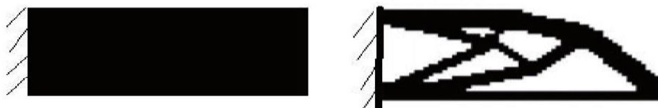
Fig. 29: Initial (left) and optimized (right) structure of a cantilever beam using a topological optimization algorithm (Chen et al., 2018)
