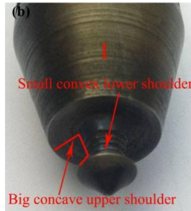
Figure 15. Bobbing tool for extruded profiles [48]
