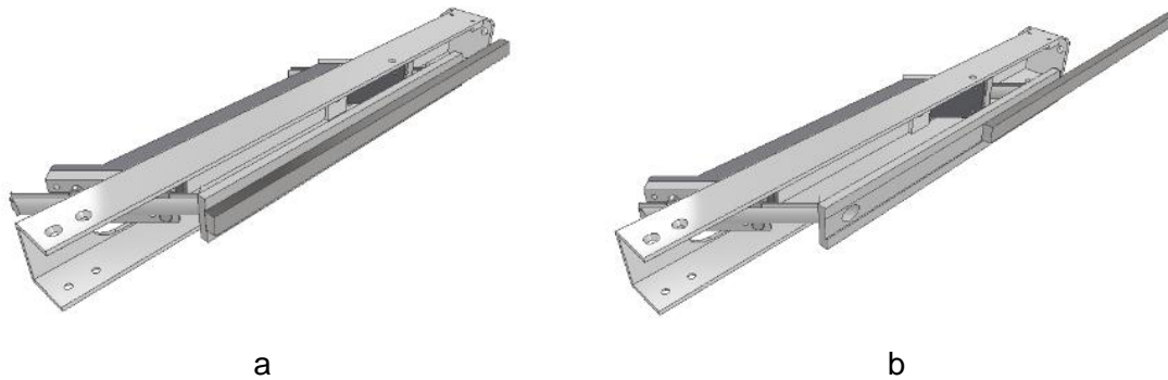
Figure 19. Displacement of the components. a) assembly when the door is closed, b) assembly when the door is open
