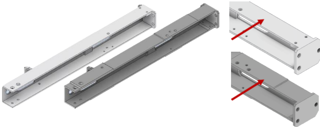
Figure 20. CAD models of the ties. At left the original, at right the locally manufactured. On the side a zoom of the differences at the ties.
