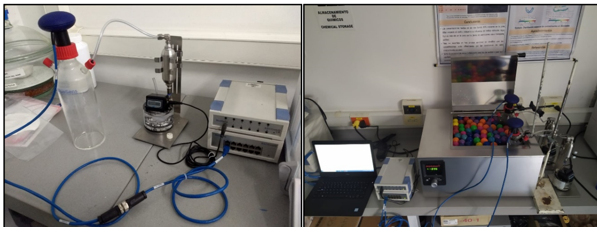
Figure. 2-6 : On-line methane measurement assay setup.
