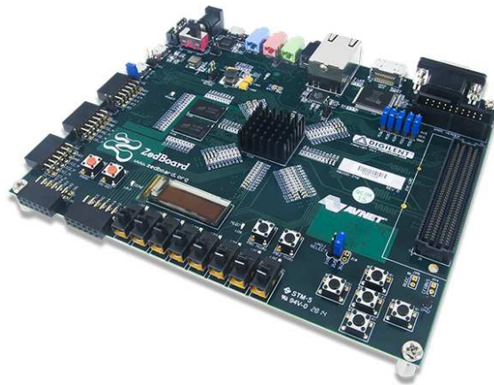
Figura 2-5.: Sistema de desarrollo ZedBoard Zynq Evaluation and Development Kit
