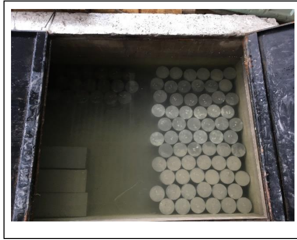
Figure 56 – Specimens in curing conditions submerged in water tank at 21°C.
