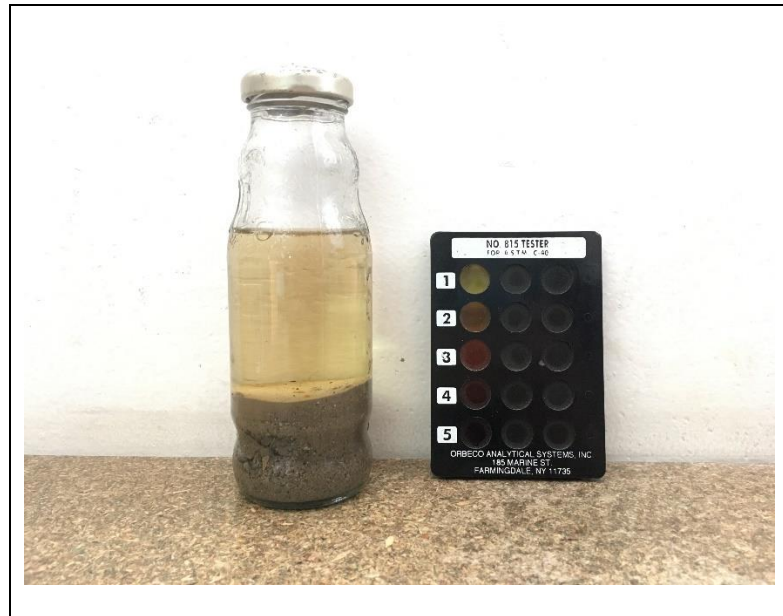
Figure 20 – Organic Impurities testing in fine natural aggregates.
