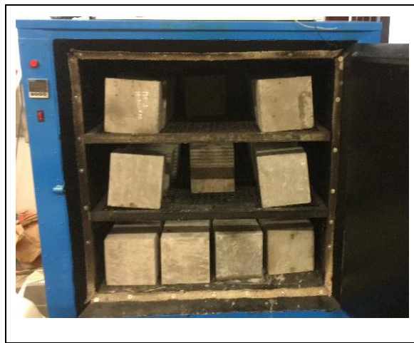
Figure 88- Cubical specimens oven-drying at 50°C for 4 days.
