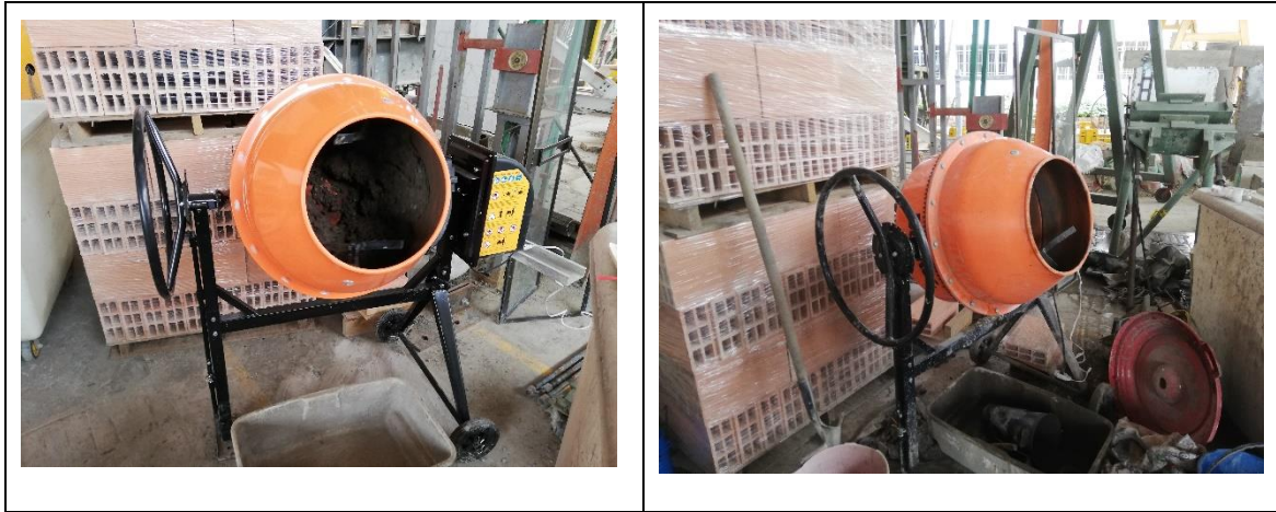
Figure 48 – Concrete mixer used in experimental program.
