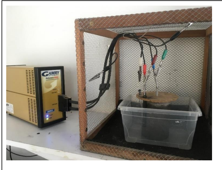
Figure 81 – Electrochemical cell for measuring polarization resistance connected to GAMRY potentiostat.
