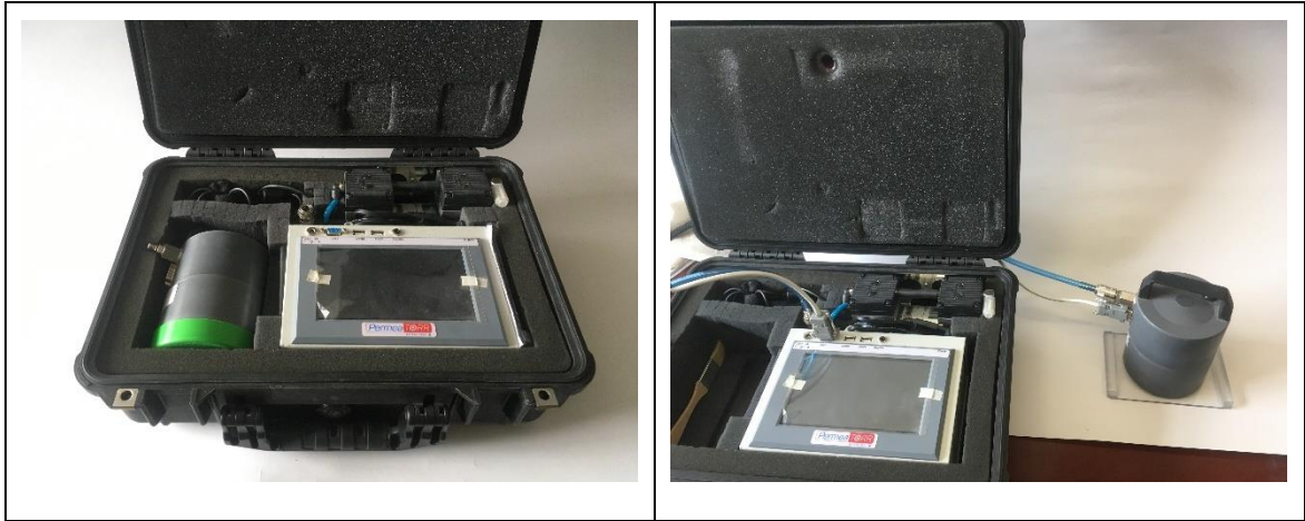
Figure 86 – PermeaTORR device used for Air-Permeability testing of concrete samples.
