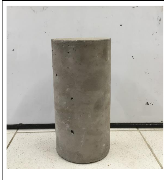
Figure 51 – Demolded cylindrical specimen used in concrete testing (4 x 8 inches – 100 x 200 mm)
