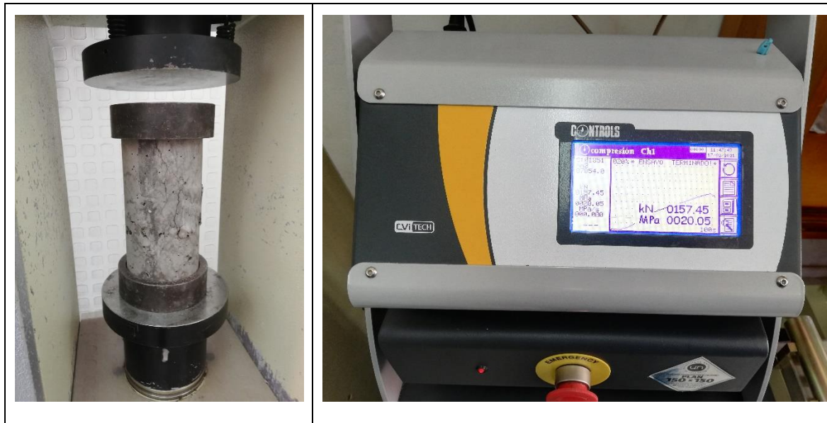
Figure 62 – Experimental setup for compressive strength testing.
