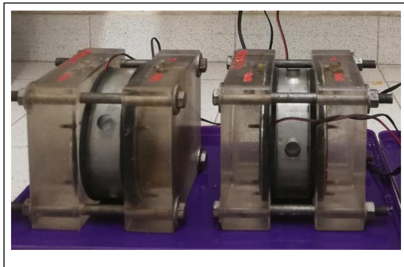
Figure 69 – Voltage cell with specimen for Rapid Chloride Penetration Test.
