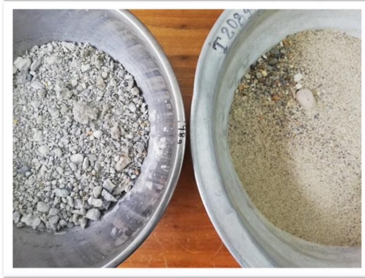
Figure 2 - Fine recycled concrete aggregates (left) and fine natural aggregates (right)
