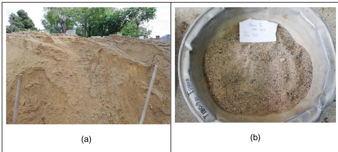
Figure 18 – Natural fine aggregates: (a). Aggregate storage at source. (b). Fine natural aggregate particles.
