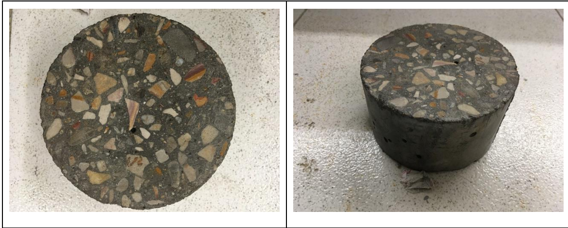
Figure 59 – Sliced 4-inch concrete cylinders.
