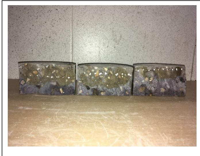
Figure 77 – Concrete specimens after spraying Silver Nitrate solution for Chloride ion indication.
