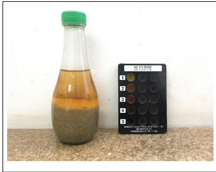
Figure 23 – Organic Impurities Testing in fine recycled aggregates.
