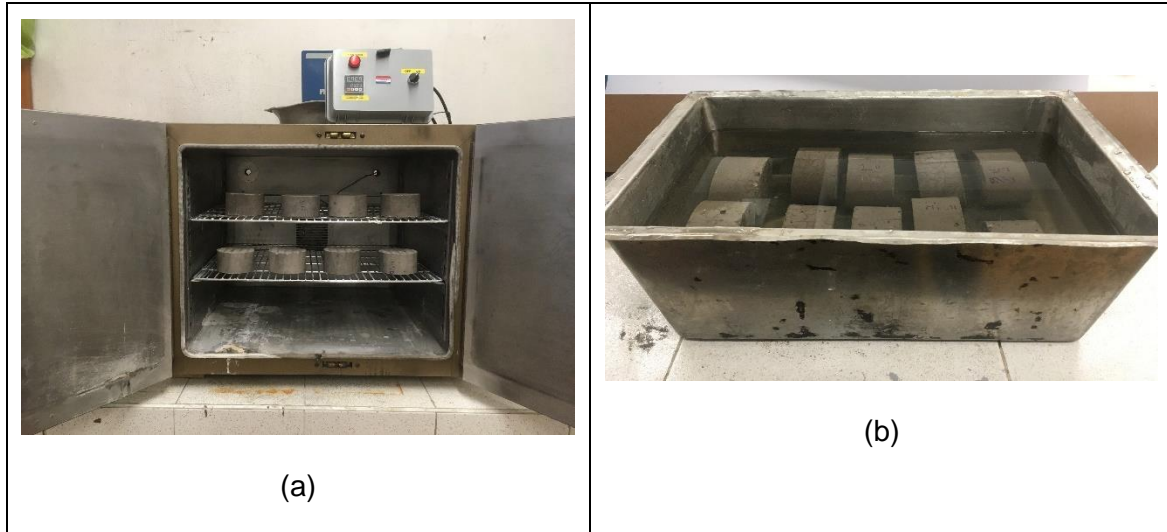
Figure 68 – (a) Concrete specimens’ oven-dried at 105°C. (b) Concrete specimens positioned on boiling reservoir.
