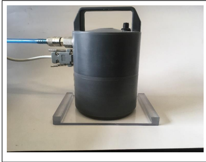
Figure 87 – (a) Calibration plate of PermeaTORR instrument. (b) Calibration process of the active cell.
