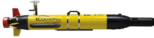
Figure 4-1: YSI Ecomapper, the underwater vehicle used to gather physicochemical data in the environment.
