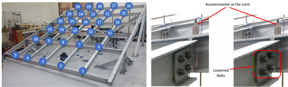
Figure 4-9: The Qatar University (QU) grandstand simulator. Source https://www.structuraldamagedetection.com/benchmark/damage/
