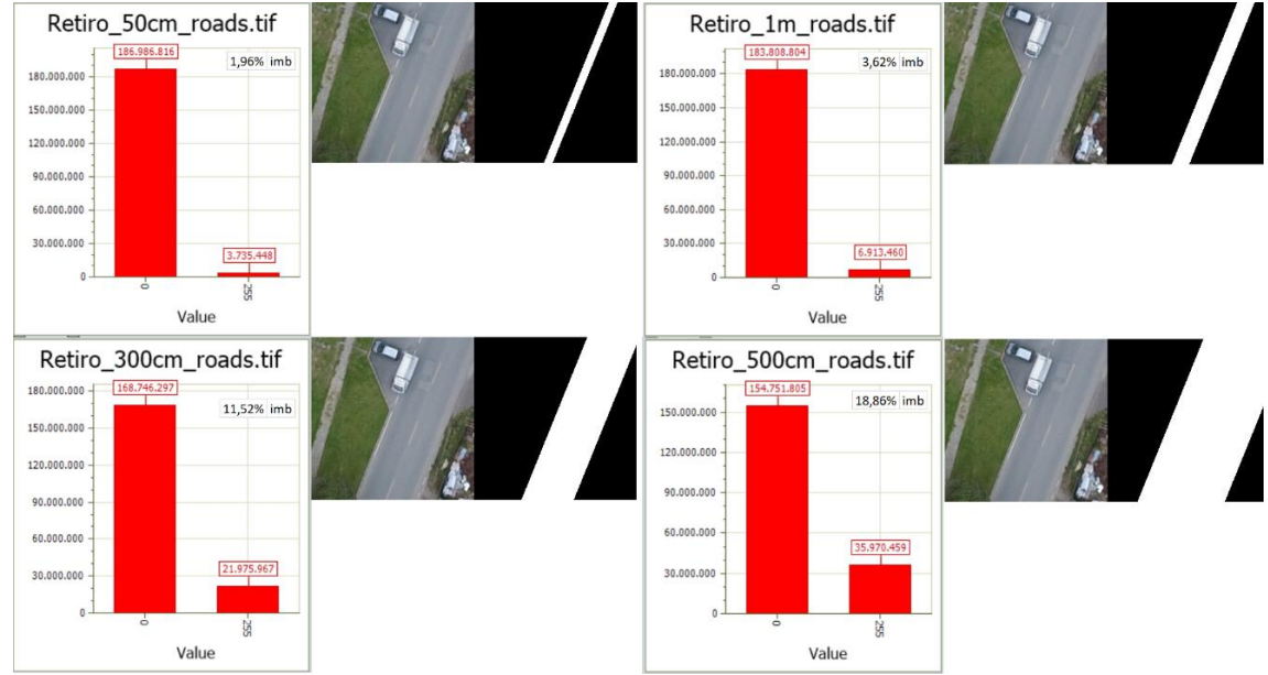
Figure 5.16. Imbalance vs buffer distance in roads. These values are averaged for the entire raster masks not yet tessellated.
