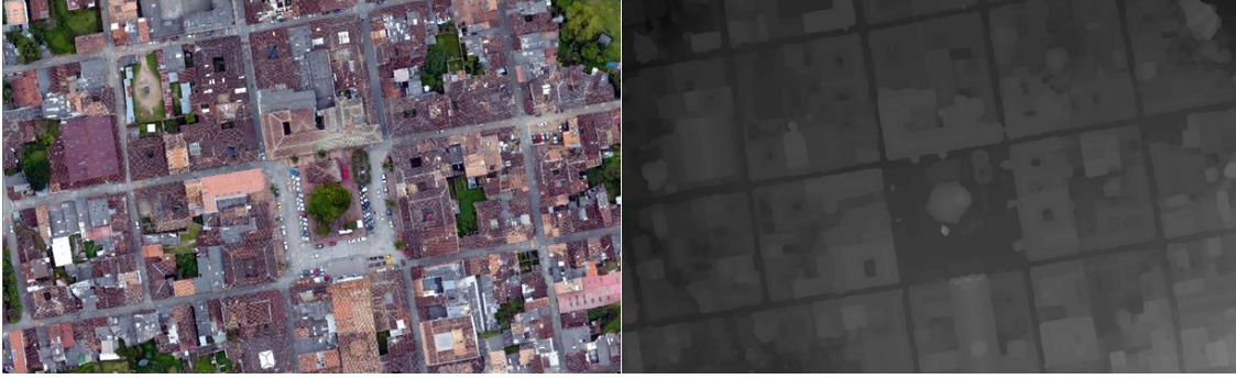
Figure 4.3. Drone orthomosaic and DSM [1] Aerial Raster Layers. This example corresponds to the urban area of El Retiro, Colombia, with a GSD of 7.09 cm/px.
