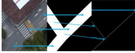
Figure 6.1. Example of a Primitive Mask for Roads. It consists of setting an optimum value for a buffer distance.
