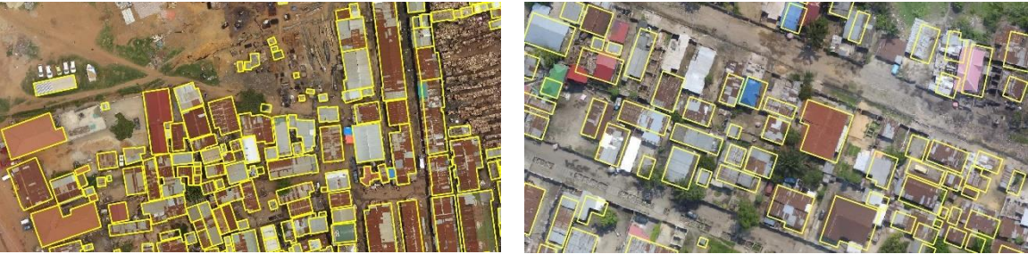
Figure A2.8. Open Cities Dataset. Quality of hand-drawn building footprint labels (alignment and completeness) can vary across or within image scenes. Examples from Challenge training dataset for Kampala, Uganda (left) and Kinshasa, Democratic Republic of the Congo (right).
