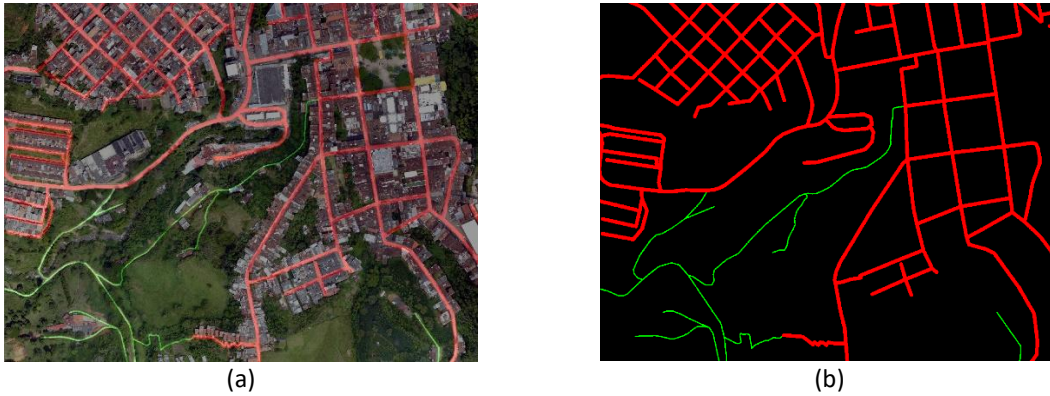
Figure 4.11. TSQS Road Dataset. (a) Orthomosaic-mask, (b) mask using attribute type of road: red color represents paved roads, green represents unpaved, and black the background class.
