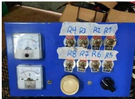
**Figura 18.** Banco de resistencias en funcionamiento
