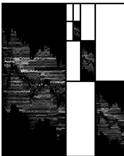
Figure 4-1.: Example of image produced by four levels of compression using haar wavelet transform.
