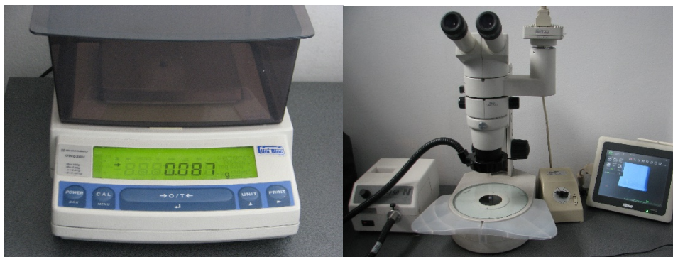
Fig. 56 Shimadzu UW620H precision balance and Nikon SMZ800 stereo microscope were used for the dimensional analysis.
