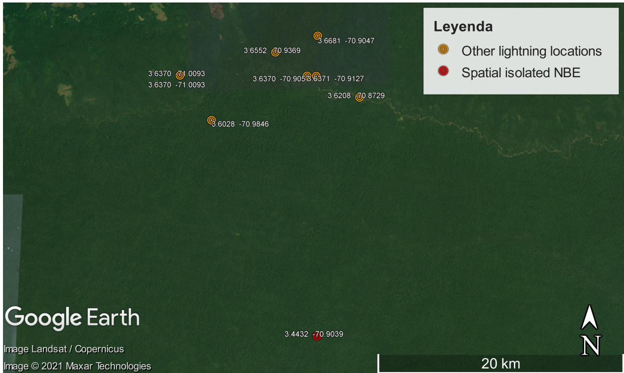
Figure 4-21.: An example of a spatial isolated NBE. The pulses were recorded on November 20, 2019, at 19:32:55 UTC. Lightning events in the figure took place for 8 seconds. The source of the emissions is approximately 350 km from the lightning station (Latitude 3^{\circ} 38' 13,2'' N, Longitude 71^{\circ} 0' 33,479 W, Puerto Gaitán, Meta). Source: Google earth V 7.3.4.8248. (November 19, 2021). Puerto Gaitán, Meta, Colombia. 3^{\circ} 38' 13,2'' N, 71^{\circ} 0' 33,479 W, Eye alt 50 km. http://www.earth.google.com .
