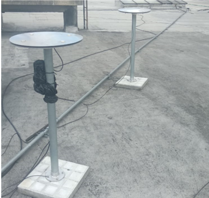
Figure 3-5.: Photograph of a pair of flat plate antennas built for this study.
