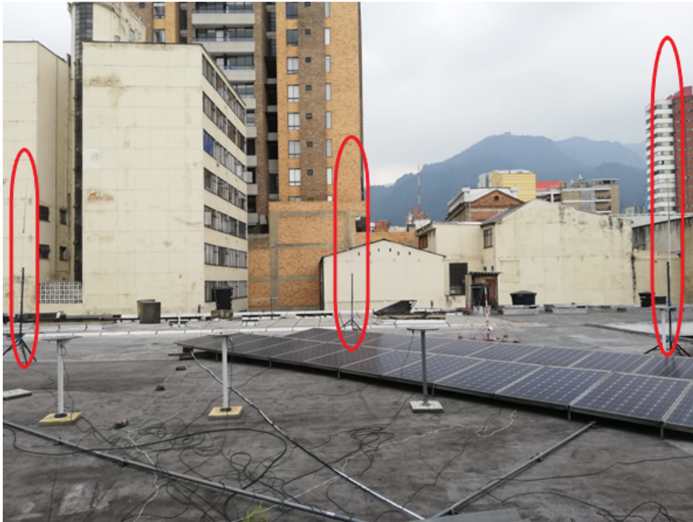
Figure 3-11.: Depiction of the broadband lightning interferometer. The separation between antennas is 10 meters and the orientation of the array is North-South, East-West.
