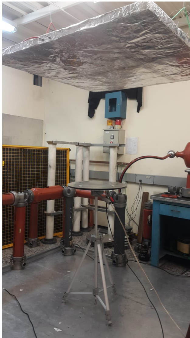
Figure 3-8.: Physical setup used in laboratory facilities to determine physical characteristics of flat plate antennas built for this study.
