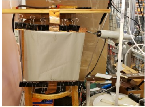
Fig. 5. Experimental assembly to fix the 30x30 \text{cm}^2 conductive fabrics test samples connected to the 10/350 \mu\text{s} LICG at KTH, Sweden [2]. Notice that in this assembly current flows from the upper to lower side in this assembly
