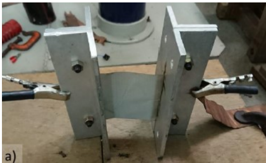
Fig. 3. Experimental assembly to fix the 10x10 \text{cm}^2 conductive fabrics test samples connected to the 8/20 \mu\text{s} LICG at the IEE-US, Brazil [8]. Notice that current flows from left to right in this assembly
