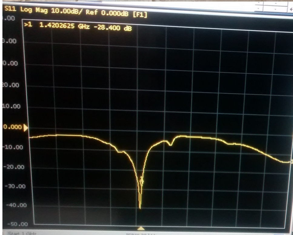
Figure 4-2.: (a) Printed Yagi-Uda Antenna, fabricated with photolithography for radio interferometer implementation. Top: Top Layer View; Bottom: Bottom Layer View. (b) Validation of Input Reflection Coefficient ( S_{11} parameter) and Bandwidth for manufactured Yagi-Uda Antenna at the Electronics Engineering Laboratory - Universidad Nacional de Colombia [11].
