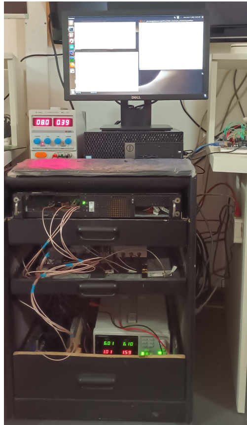
Figure 4-16.: Implemented Correlation and Down-conversion stages, along with the control system for the instrument.
