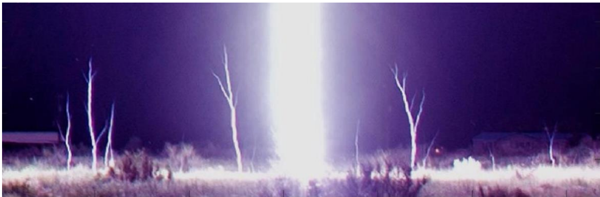
Figure 2-7. Image magnification of a lightning attachment photograph taken in southern New Mexico, USA, showing at least 12 unconnected upward leaders in the form of branches emanating from the ground. Source: [75].
