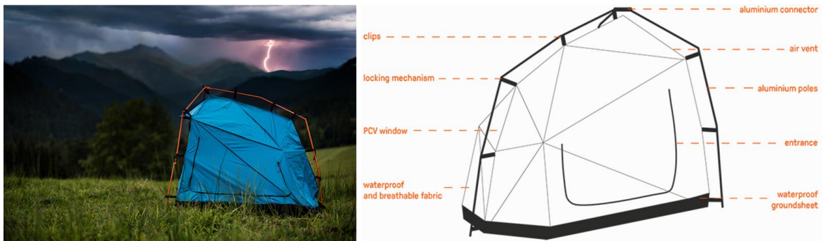
Figure 3-5. Lightning protection tent designed by Kamila Jania and tested at the Warsaw University of Technology, that consider the conductive structure as a measure of protection. Source: https://www.designboom.com/design/kama-jania-bolt-tents-lightning-strike-protection-01-21-2016/
