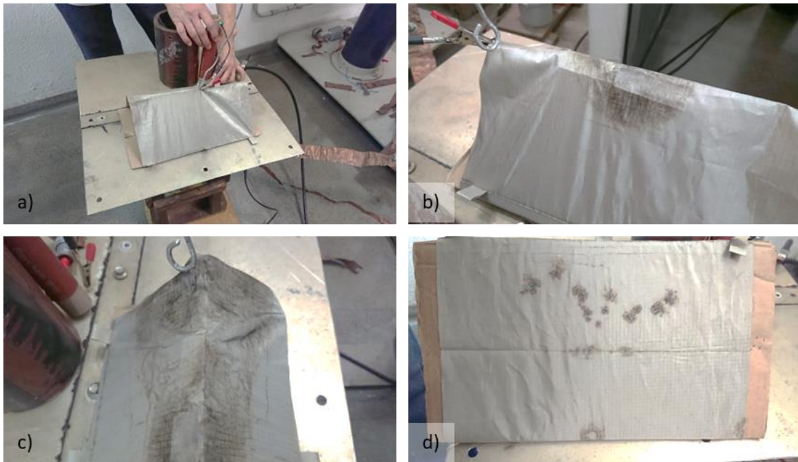
Figure 4-24. Images of 1:10 scaled A-shape tent model during the test process, a) previous to the first 20 kA test at the center of the ridge, b) after the first test with the notorious concentric mark, c) after the second 20 kA test at one end of the ridge showing the surface marks around the entry points, and d) the model base after the two current impulses.
