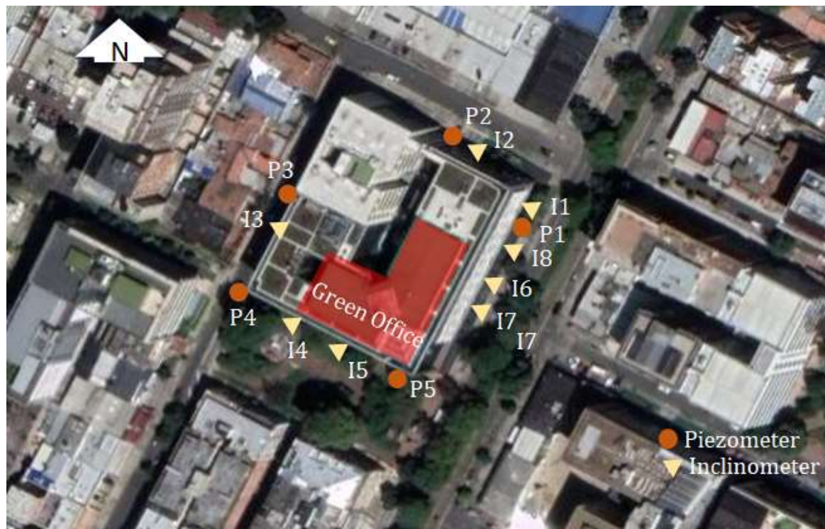
Figure 5-6. Location of inclinometers and Casagrande piezometers installed before the construction stage (Modified from Google Earth 2022).
