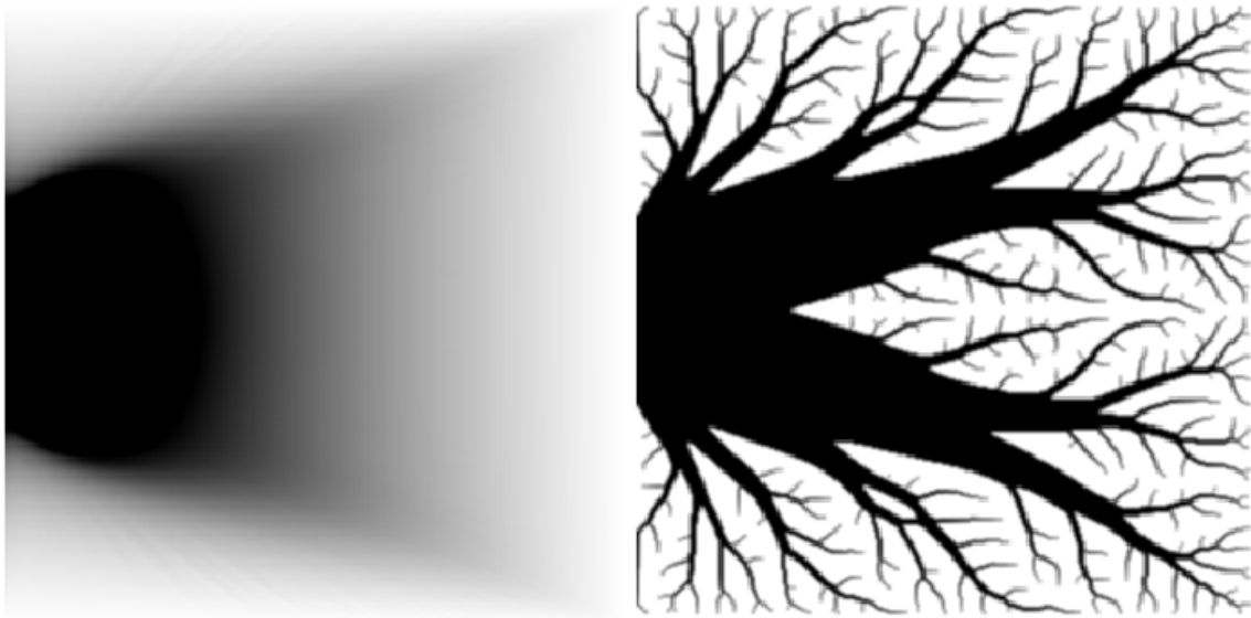
(a) Area-to-point problem without penalization, p = 1 . Compliance c/c_0 = 1.000 (b) Area-to-point problem with penalization, p = 3 and without continuation. Compliance c/c_0 = 1.161
