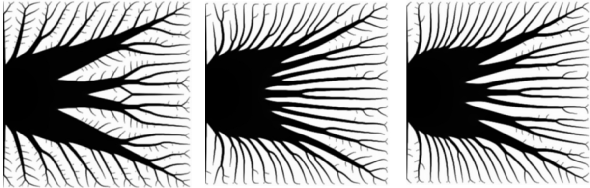
(a) Continuation, step 2 \cdot 10^{-2} . No regularization. c/c_0 = 1.157 (b) No continuation. c_{r-max} = c_0 \cdot 1.30 \cdot 10^7 c/c_0 = 1.131 (c) Continuation, step 2 \cdot 10^{-2} . c_{r-max} = c_0 \cdot 3.84 \cdot 10^6 c/c_0 = 1.138
