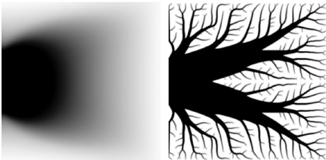
(a) Solution without penalization, p = 1 . Compliance c/c_0 = 1.000 (b) Penalization p = 3 and no continuation. Compliance c/c_0 = 1.186
