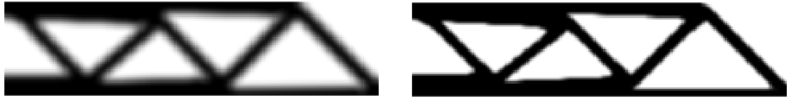
(a) Result of the first phase with r = 5 . Compliance c/c_0 = 1.140 (b) Final result with radius r = 2 . Compliance c/c_0 = 1.114 .
