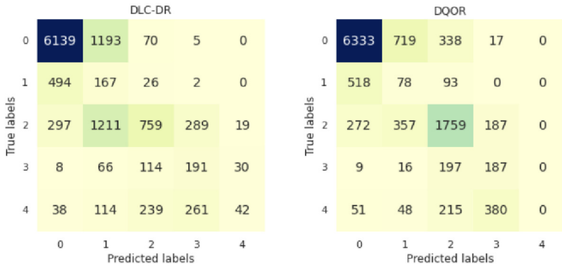
Figure 6-8.: Confusion matrices of the predictions of DLC-DR (left) and DQOR (right) in the EyePACS-b test partition.
