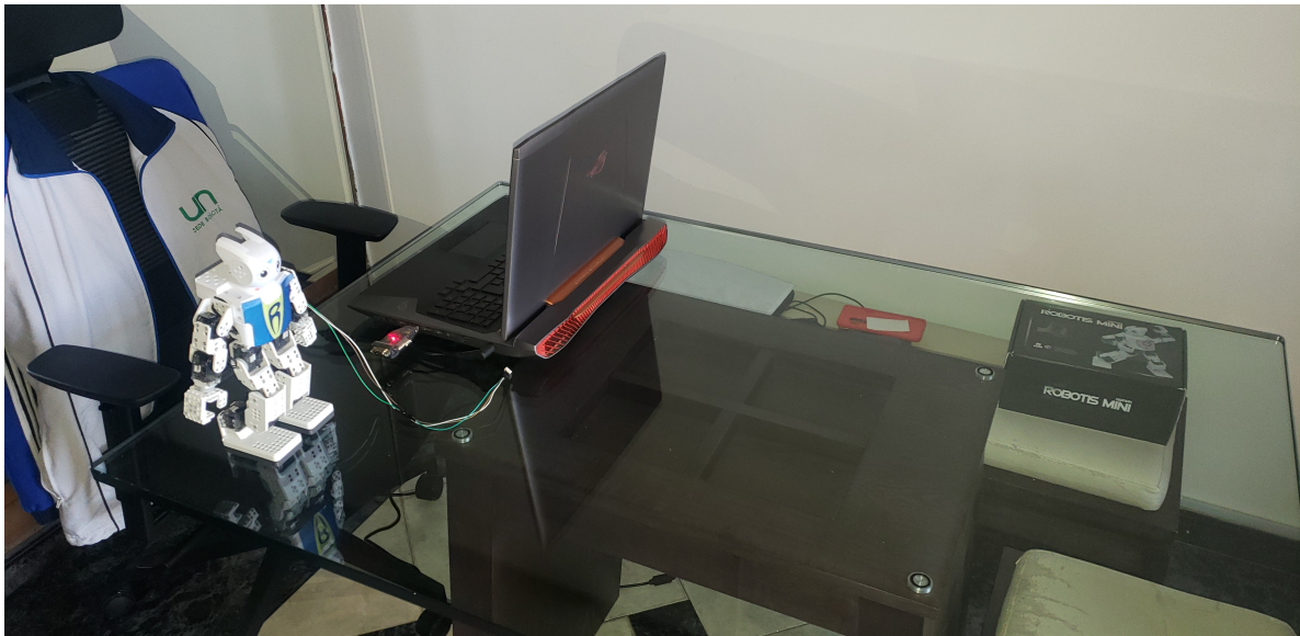
Figure 5-4.: Experiments setup for the physical experiments. The walking surface corresponds to a glass table, and the data wire (connected to Darwin's arm) is held next to the robot to avoid interfering with the gait.
