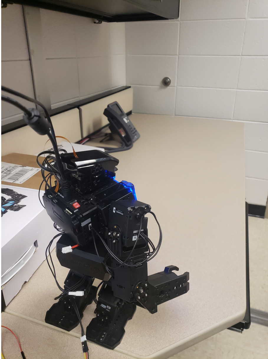
Figure 5-6.: Experiments setup for the physical experiments. The walking surface corresponds to a wood office desktop, and the power wire is held over the robot, avoiding interfering with the gait.
