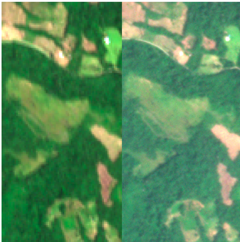
Figure 3-4: Comparison of resolution between Sentinel-2 (left) and Planet (right) imagery Source: Author's own
