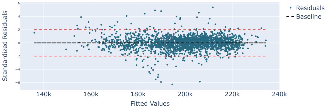
Figure 3-15.: Standardized residuals vs fitted values for the multiple linear model constructed.
