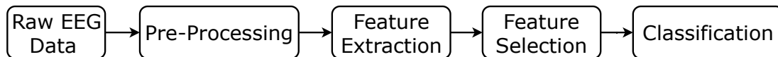
Figure 1-1. The diagram depicts the typical signal processing steps involved in an EEG-based system for MI.
