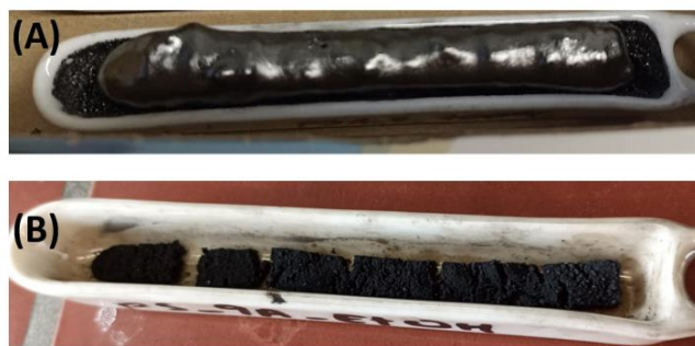
Figure 2-17. Product of carbonization of expanded starch: without doping with acid (A) and with doping with acid (B).
