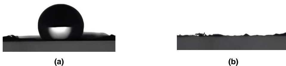
Figure 5 - 10 The wettability characteristics of the optimum PPy-PCL scaffold at (a) 0 s and (b) 1 s, respectively, illustrate that water has completely permeated the scaffold.
