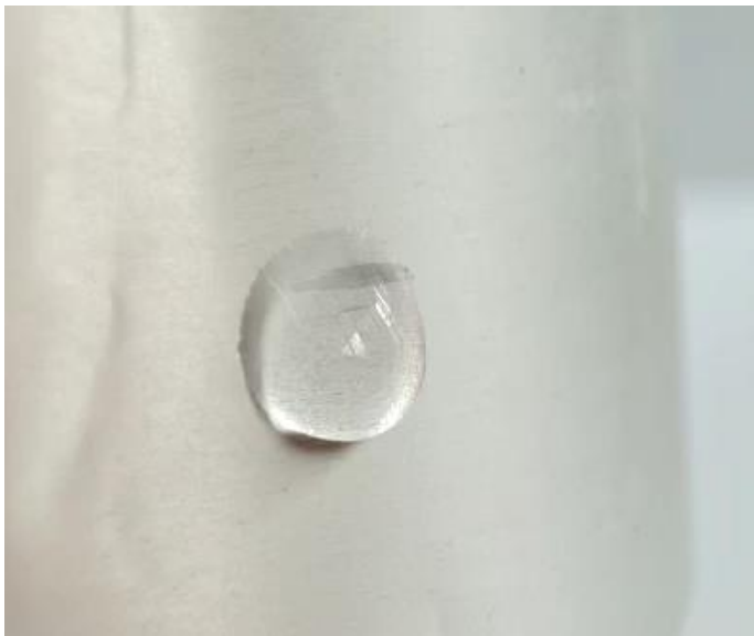
Figure 4 - 5 Contact angle of the PCL+PPy scaffold.
