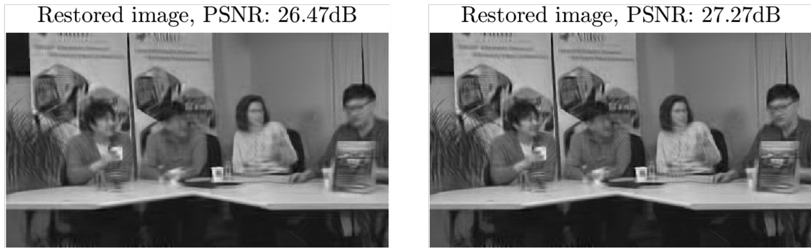
Figure 5-4: Frame restoration QP=185 , block-size = 16 \times 16 , nonzeros \in \{2, 4\} , overlapping factor=4.
