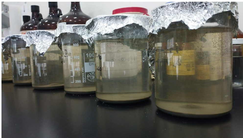
Figure 3. Density separation of MPs using NaCl saturated solution. The sediment can be seen on the bottom of the beakers, while MPs remain on the surface.
