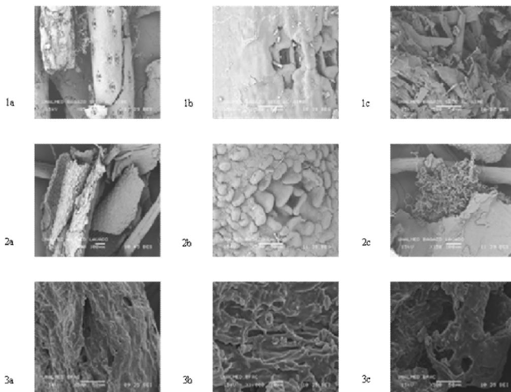
**Fig. 1** SEM photographs of Raw Figue's Bagasse, RFB (1a-1c); Washed Figue's Bagasse, WFB (2a-2c); and Activated Figue's Bagasse, ACFB (3a-3c).
