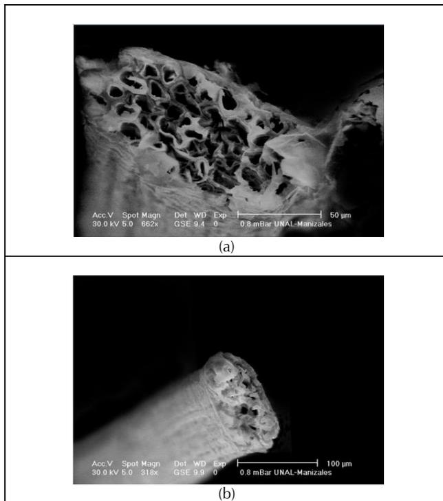
Figure 3. Angular view of surface fractured of (a) untreated banana fiber and (b) treated banana fiber.
