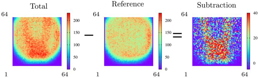
FIGURE 1. *Experimental image of a steel pliers behind an aluminum plate with 1 cm thickness. The subtraction between the total and the reference image is the contribution to the total image from the pliers.*
