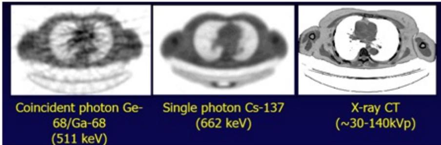
FIGURE 3. Evolution in attenuation correction maps from left to right, line source  $^{68}\text{Ge}$  transmission (5 min/15 cm),  $^{137}\text{Cs}$  point source (2 min/15 cm) and CT imaging (1 min/100 cm).
