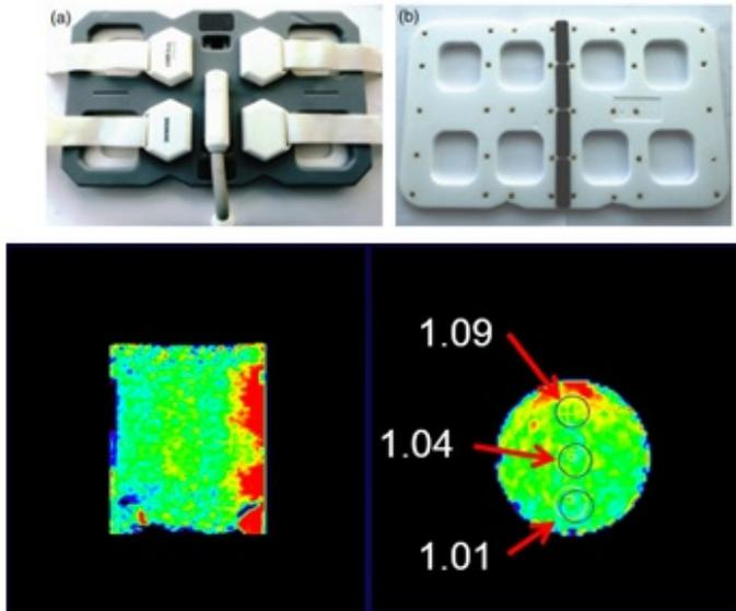
FIGURE 8. Chest flexible phased array coil used for body PETMR imaging (top), and effect of these coil of PET accuracy (bottom).
